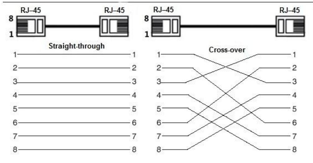
The cable connection of RJ-45 connector conforms to the standard 568B (1-orange white, 2-orange, 3-green white, 4-blue, 5-blue white, 6-green, 7-brown white, 8-brown).
