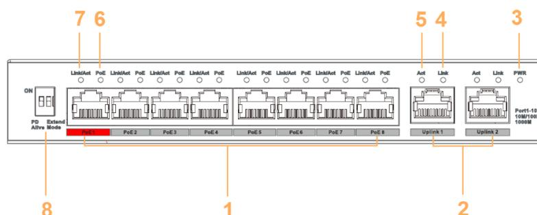
The following are all the ports and indicators on the front panel of the 4/8-port unmanaged desktop switch. The actual device may only have a part of them. Refer to the table below for the contents of the actual device panel.
