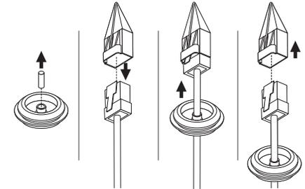
4. Insert the cable bushing into the groove of the housing installation unit.
