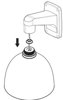
5. Attach the housing to the bracket by turning it clockwise.
