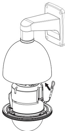
7. Connect the network cable to the network terminal.
