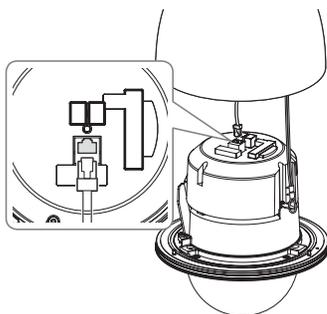
8. Align the holes of the camera body and the housing and turn them slightly.
