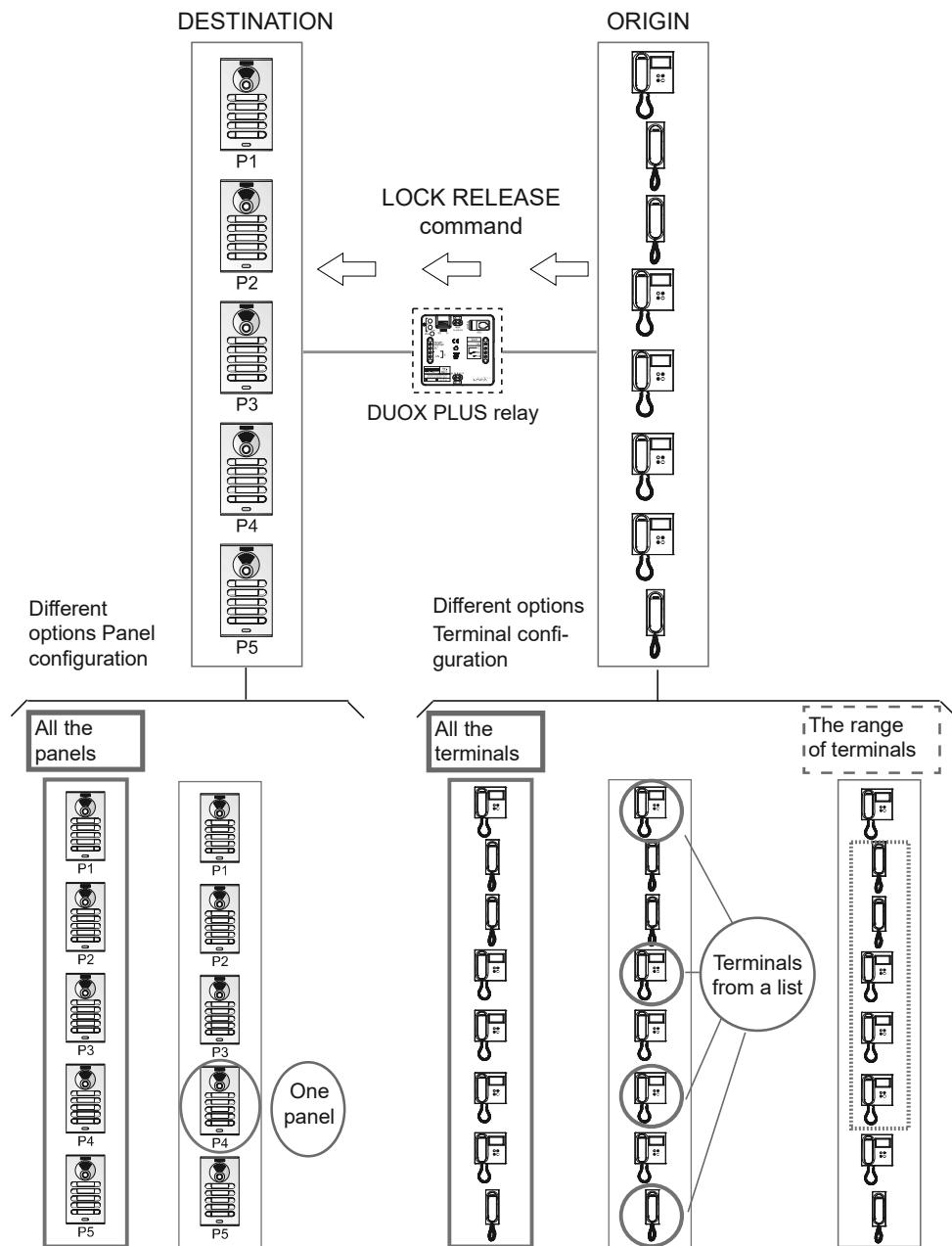
**Function configuration.****First step: Configure the command and panel.**
