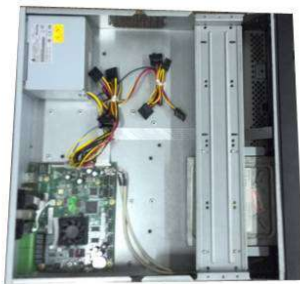
Figure 3-45 Put bracket back
