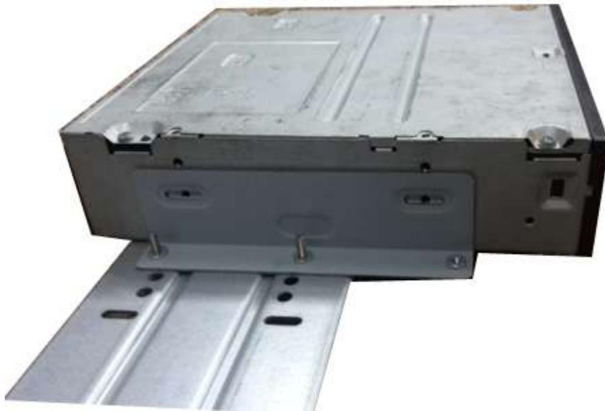
Figure 3-43 Install SATA burner
