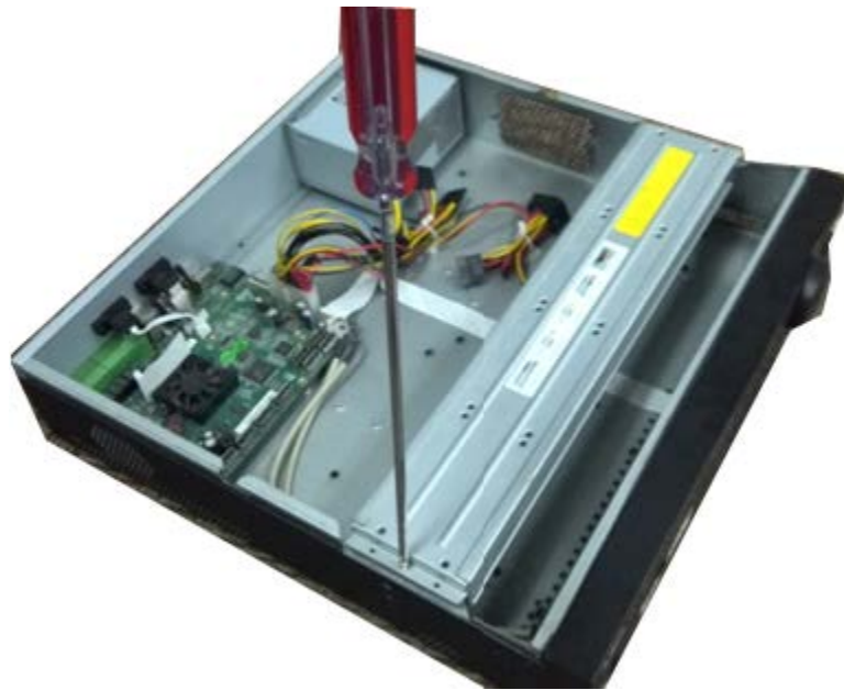
Figure 3-37 Open the top cover
