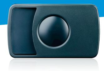
The LEGIC Booster Ultimate is a vehicle and driver identification tag. This patented solution ensures that a vehicle can only get access to a secured area when driven by an authorized driver. The LEGIC Booster Ultimate is used in combination with (existing) LEGIC smart cards. Based on semi active RFID technology, the LEGIC Booster Ultimate is identified up to 12 meters\* (40 feet) with the TRANSIT Ultimate reader.
