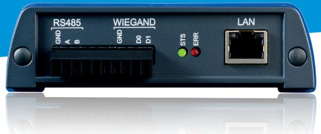
The Wiegand Interface Module ensures an easy integration of the ANPR Access (HD) into any existing or new access control panel that support Wiegand. This module converts license plate numbers that are captured by the ANPR Access (HD) into Wiegand ID strings.
