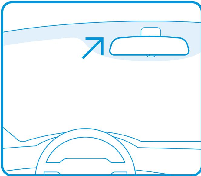
Determine the position of the Windshield Tag on the inside of the vehicle's window\*.
