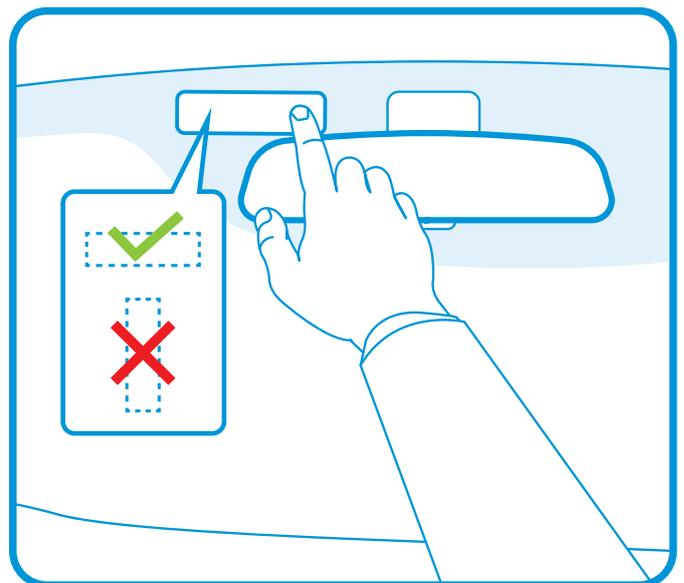
Ensure that the tag is positioned horizontally and in line of sight of the uPASS Reach reader.
