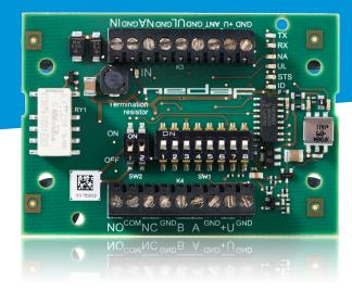
The TCC270 enables uPASS Access (or any other Nedap reader with RF output) to operate in a mode that is compatible with TRANSIT and uPASS Reach readers.
