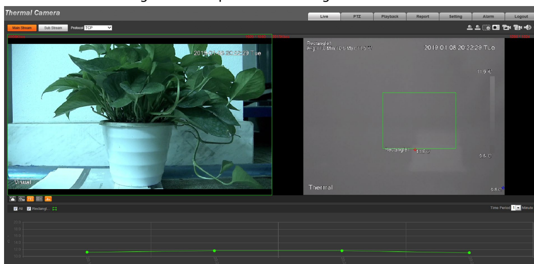
Figure 4-5 Temperature recording area
