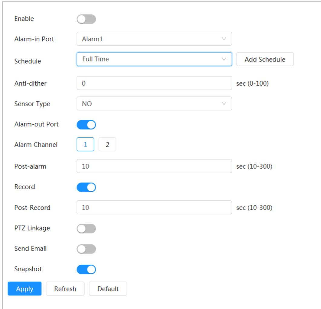
**Step 3** Select an alarm-in port and a sensor type.
