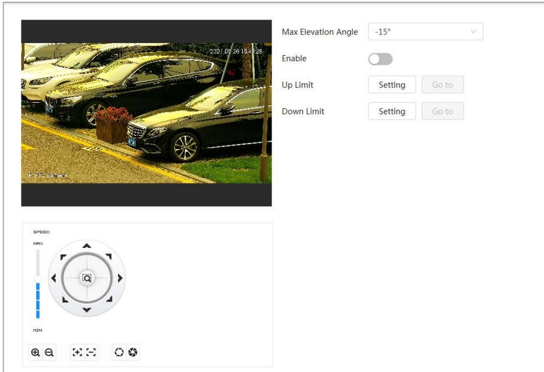
**Step 5** Select the elevation value from the drop-down list of **Max Elevation Angle**.
