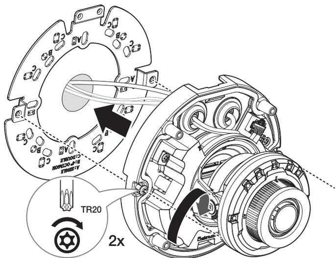
10. Adjust the lens to the desired direction with reference to "Adjusting the monitoring direction for the camera" section. (page 18)
