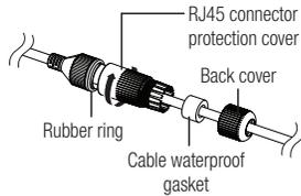
5. Assemble by rotating RJ45 protection cover and back cover clockwise (Follow the arrow).
