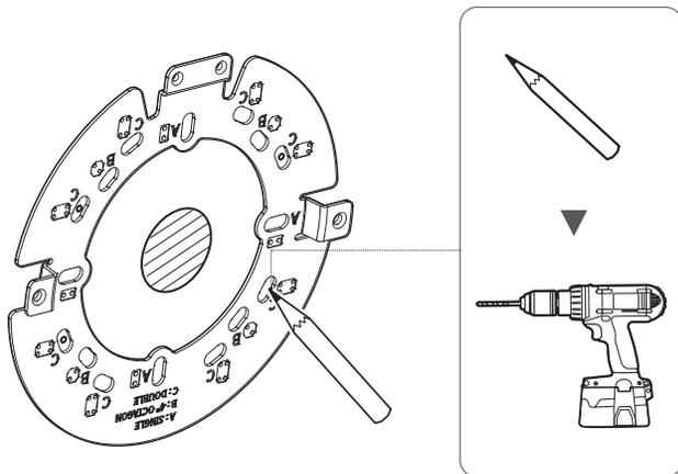
2. Fix the mount plate using appropriate screws.
