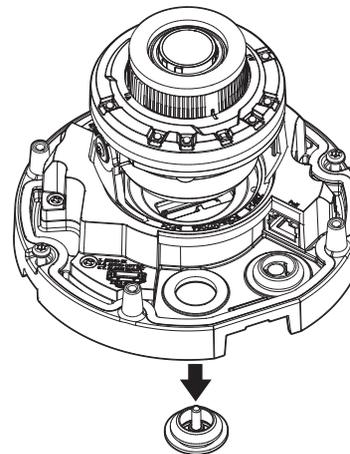
2. Remove the protruding part of the 1-hole cable bushing that was removed from the camera body.
