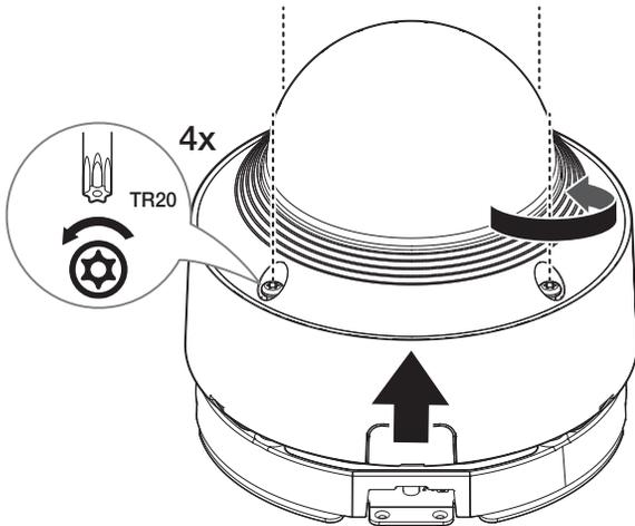
2. Remove the camera body by turning the mount plate fastening screws counterclockwise.
