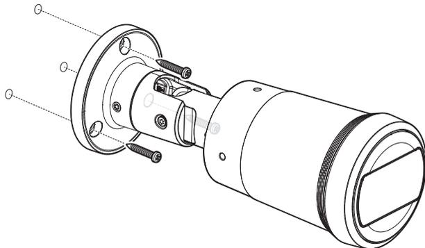
4. Loosen the fixing screws of each control part to adjust the monitoring direction of the camera.
