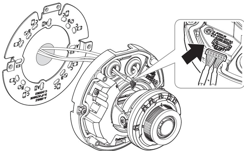
9. Join the camera body with the mount plate.
