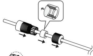
2. Connect the LAN connector (male) to the cable.
