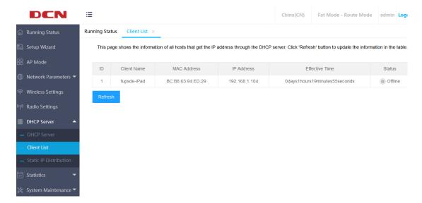
Client Name: This field displays the client name that has obtained the IP address.
