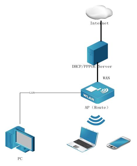
On the WAN side of the AP, set the WAN port address through PPPoE, DHCP, or static address, and then connect to the Internet or other network through the gateway device. LAN and WLAN constitute a private subnet. Devices on this network apply to the AP for dynamic or static IP addresses through DHCP.
