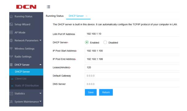
IP Pool Start Address and IP Pool End Address: These two items are the start address and end address when the DHCP server automatically allocates IP addresses. After setting these two items, the IP address obtained by the intranet host will be between these two addresses.
