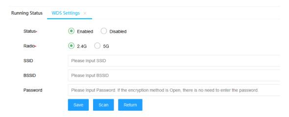
If you want to manually enter the information of the target wireless network or the target wireless network is a hidden network, you can directly enter the related wireless network information and save it.
