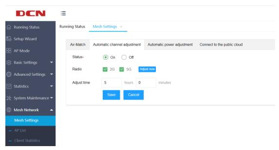
The automatic power adjustment function is on by default. The AP of mesh network can automatically adjust the power according to the set adjustment cycle, as shown in the following figure:
