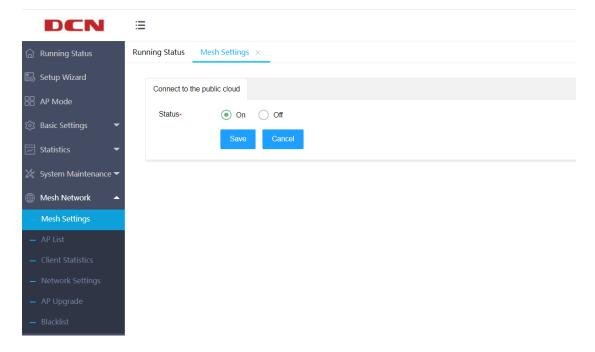
• When mesh is Master mode, it is connected to the public cloud by default. At this time, the Master AP of mesh will be online in the public cloud. When the connection to the public cloud is enabled, some local configuration functions of the mesh network will be turned off, and the configuration will be distributed by the public cloud. After the "Connect to the public cloud" status is configured as off, the AP can configure other global functions.
