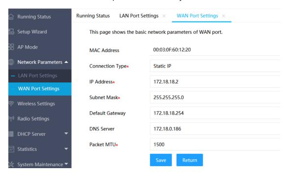
DNS Server: This shows the DNS server address automatically obtained from the ISP.
