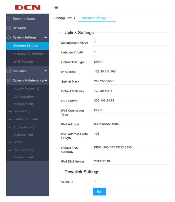
If you need to modify the related setting of the uplink port, you can click the "Edit" at the bottom of the interface to edit setting, where you can set the AP wired VLAN and the IP address configuration mode of the AP. As following:
