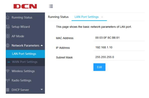
MAC Address: The MAC address of the AP to the LAN is used to identify the local area network and cannot be changed.
