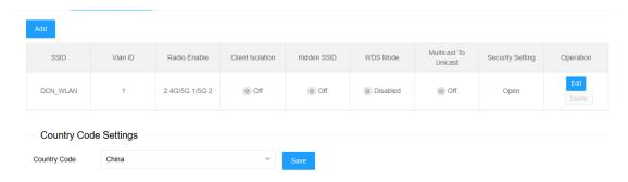
If you need to create a new wireless network, you can click "Add" and enter the corresponding parameters, as shown below:
