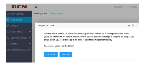
If you want to use the wizard, you can click "Next Step" to enter the "Setup Wizard-Manage IP Settings" interface, where you can configure the AP's IP (v6) address connection method to be dynamic or static, as shown below:
