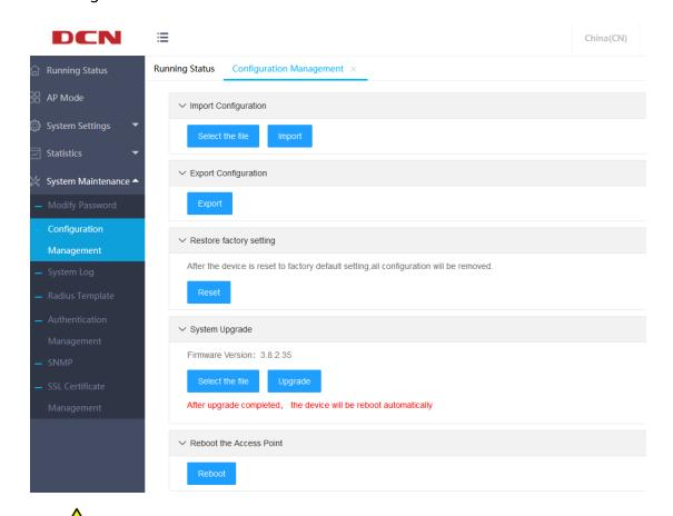
After the device is reset to factory default, all configurations will be deleted and restored to FIT mode.
