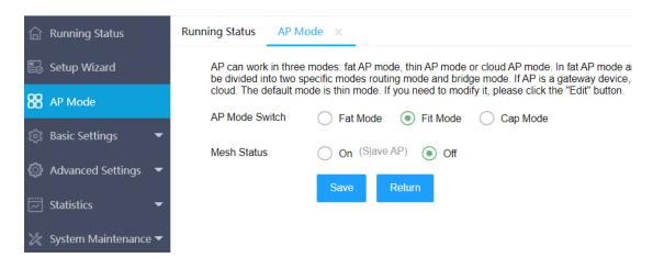
Click the Edit button on this page to edit the mesh status of the AP as "on (slave AP)". After saving the configuration, the AP will automatically restart. After restarting, the AP will switch to the mesh slave mode. At this time, the AP can only go online in the mesh master AP, and the wireless configuration and other contents are uniformly distributed through the mesh master AP (CAP).
