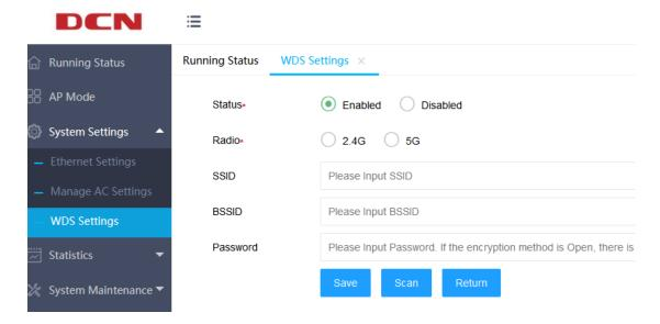
If you want to manually enter the information of the target wireless network or the target wireless network is a hidden network, you can directly enter the corresponding wireless network information and save it.
