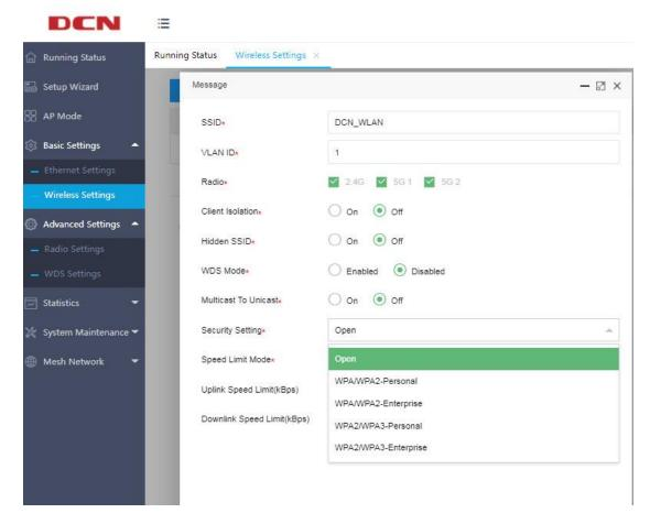
The OPEN or WPA3-Open-Transition mode does not need to set a password, and the wireless client can directly access;
