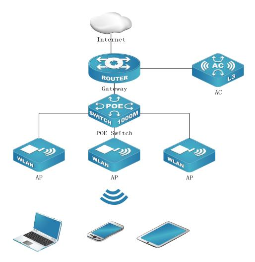
The AP is shipped in FIT AP mode by default. You can also switch to FIT AP mode by restoring the factory setting or following the instructions in the AP mode chapter. The wireless configuration of the FIT mode is operated uniformly through the AC. For details about this part, please refer to the DCN related AC operation manual. Here, the AP's wired configuration, AC address setting, WDS configuration, and system management are mainly introduced.
