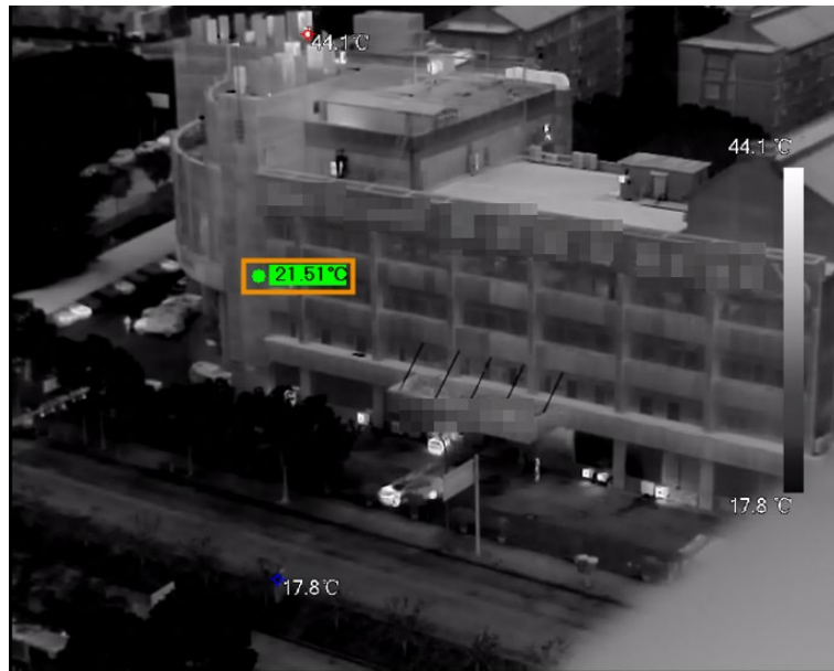
Figure 4-6 Real-time spot temperature measurement
