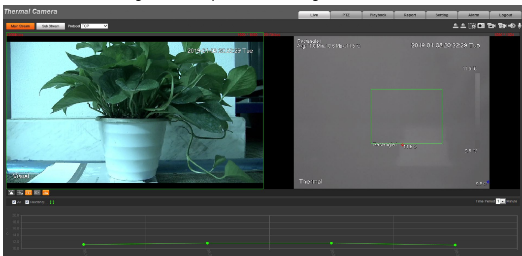
Figure 4-5 Temperature recording area
