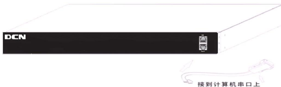
Fig 2-3 Connecting Console to switch
