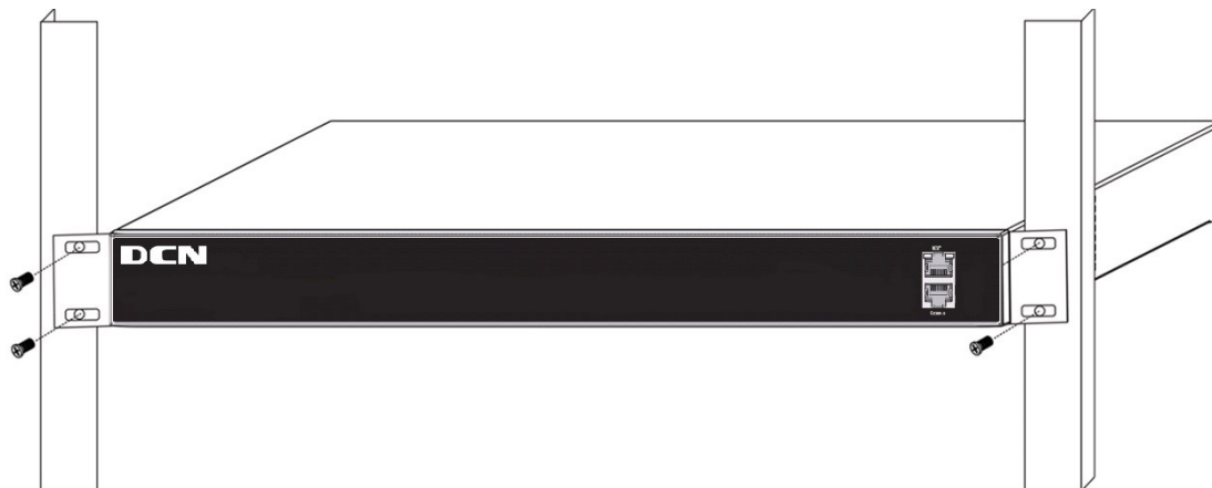
Figure 2-2 The figure of switch installing on the rack by using the front and back horn iron Caution!
