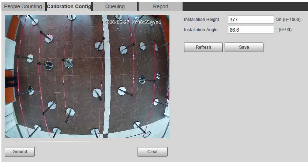
Figure 5-67 Calibration configuration (stereo analysis)
