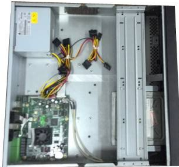
Figure 3-45 Put bracket back
