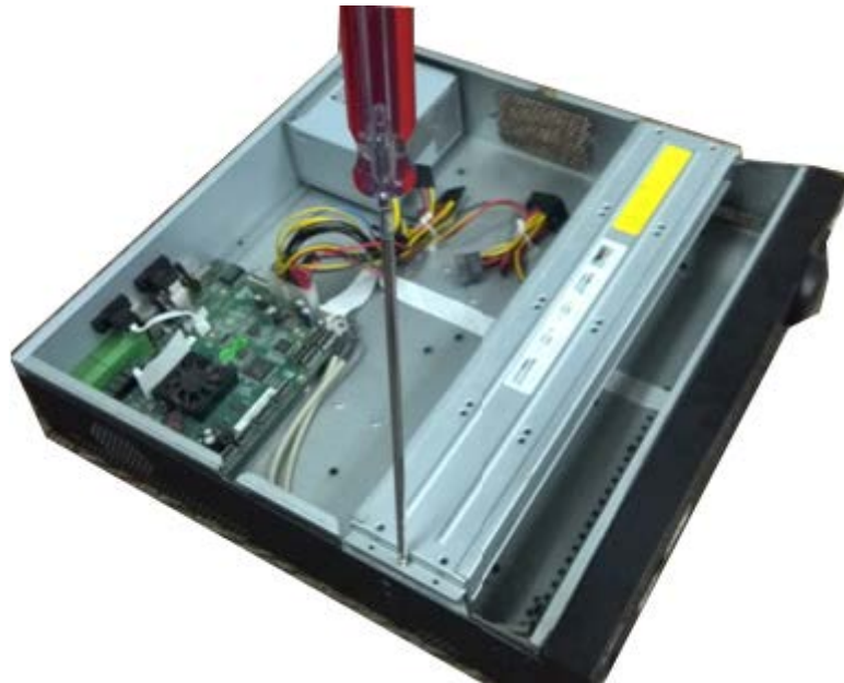
Figure 3-37 Open the top cover
