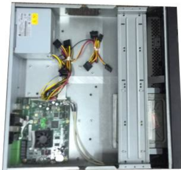
Figure 3-45 Put bracket back
