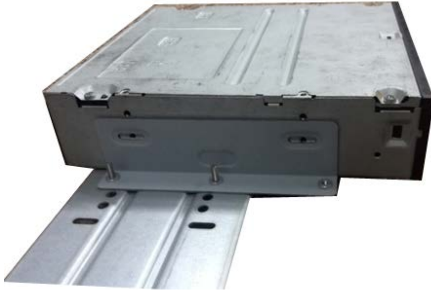
Figure 3-43 Install SATA burner
