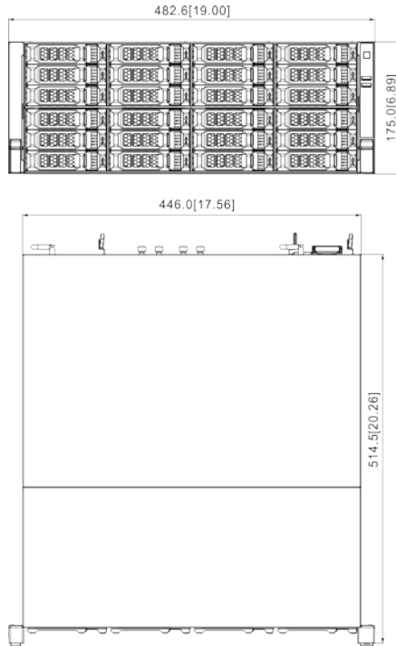
Figure 2-32 Dimensions without LCD (mm [inch])
