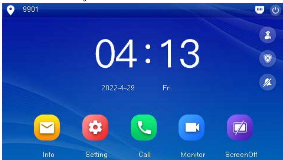
Figure 4-7 VTH main interface
