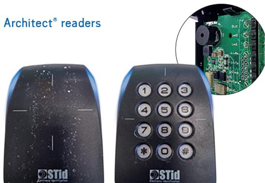
No deposit or oxidation was found on the antenna or keypad ribbon cables.
