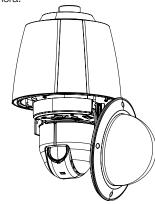
8. After confirming that the unit has been installed properly, attach the housing cover and tighten it firmly using 4 screws.
