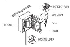
10. Fasten the door to the housing using a hexagonal wrench. (Tighten the screws while pressing the door with your hand as shown in the image below. Then tighten each of the screws a little at a time to make sure that the door is tightly pressed to the housing.)
