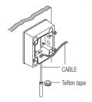
8. Install the power adaptor and media converter using the bracket adaptor, and connect the external cable.
