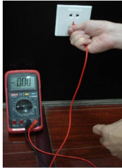
Appendix Figure 7-5 Check earth cable connection
