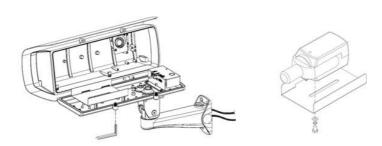
• Use 5mm wrench, open the housing top part.Remove the camera plate, Install the camera on the camera plate and screw up.Check the lens and focus and Close the housing top part and screw up tightly.
