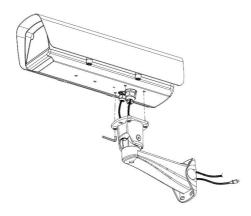
• Use 5mm wrench, Install the bracket on the camera mount part and screw up tightly
