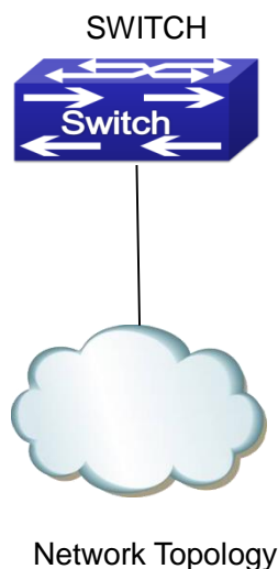
Figure 2-3 Typical example of port loopback detection
