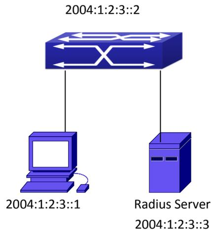
Figure 5-23 The Topology of IPv6 RADIUS configuration
