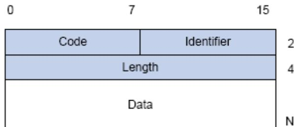
Figure 5-4 the Format of EAP Data Packets
