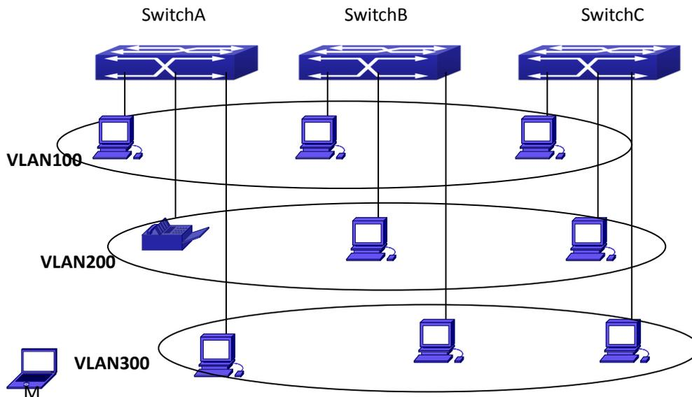
Figure 2-26 Typical topology application of dynamic VLAN
