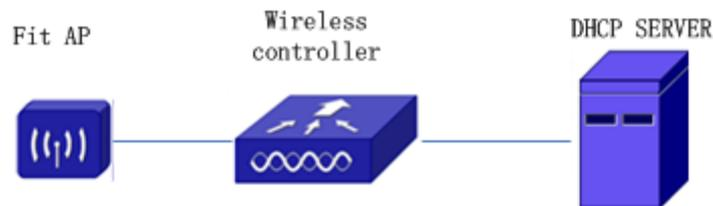
Figure 3-13 Typical DHCP option 60 and option 43 topology
