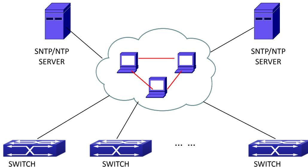
Figure 8-2 Typical SNTP Configuration
