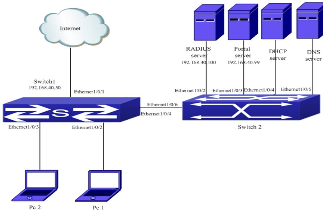
Figure 5-31 Automatic Page Pushing after Successful Authentication Configuration
