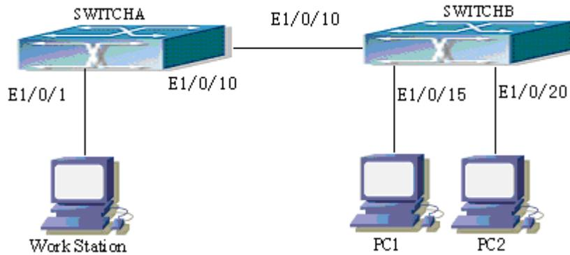
Figure 4-4 Function configuration of the Multicast VLAN
