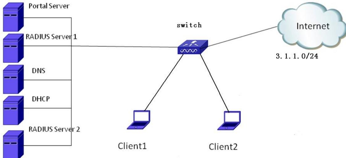
Figure 5-30 Authentication White-list function configuration
