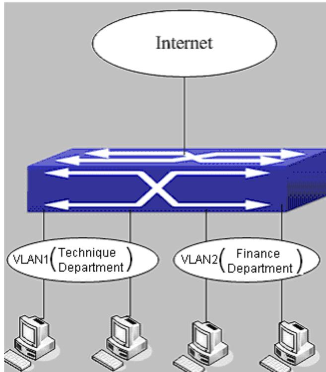
Figure 5-26 VLAN-ACL configuration example
