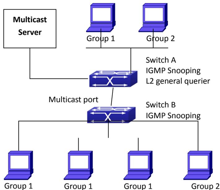
Figure 4-2 The switches as IGMP Queries
