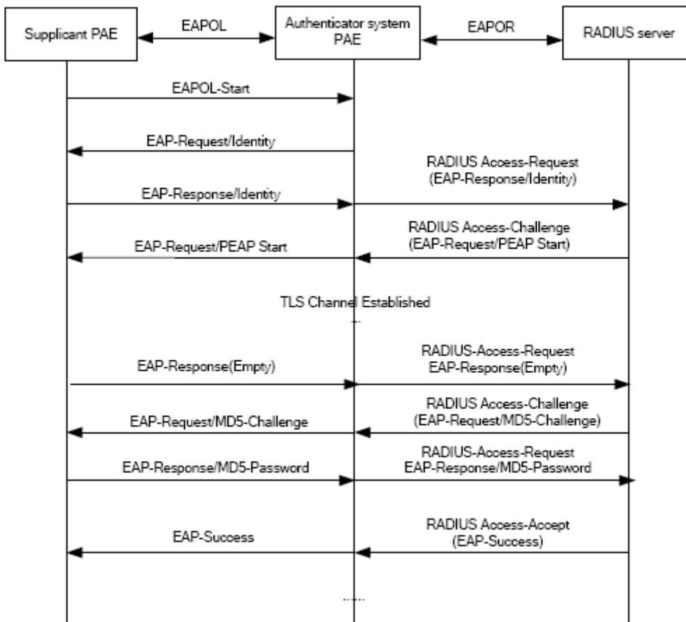
Figure 5-11 the Authentication Flow of 802.1x PEAP
