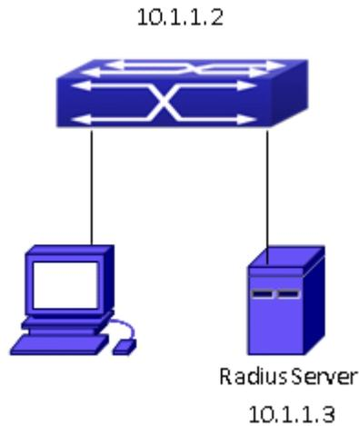
Figure 4-3 IGMP Snooping Authentication
