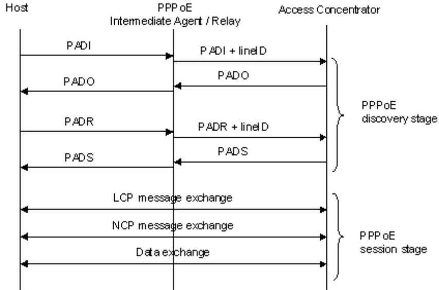
Figure 5-37 PoE IA protocol exchange process
