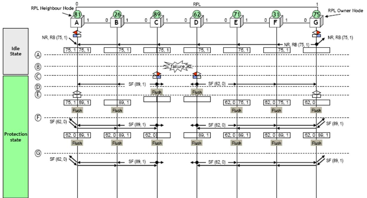
Figure 6-6 single-link fault
