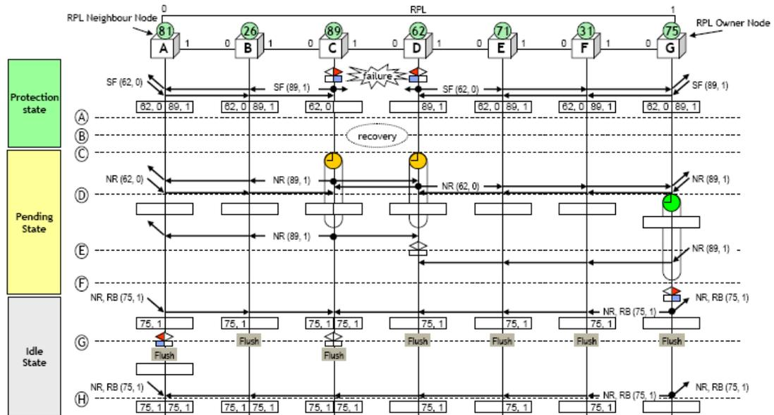
Figure 6-7 Revertive switch fault restoration of single link
