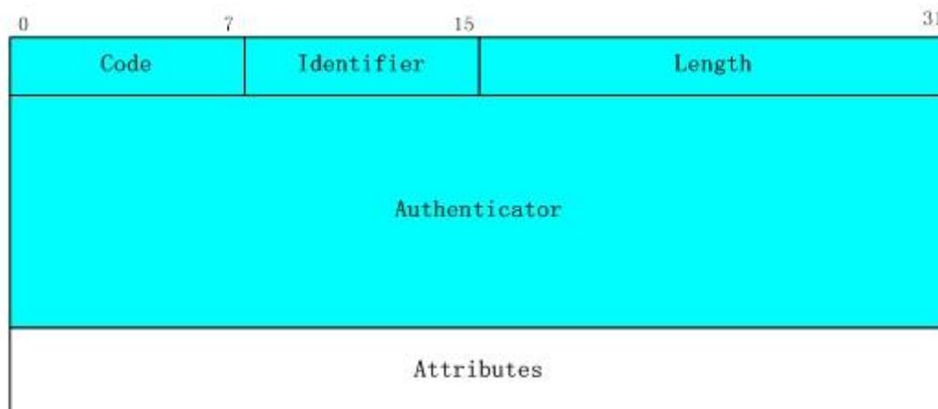
Figure 5-21 Message structure for RADIUS
