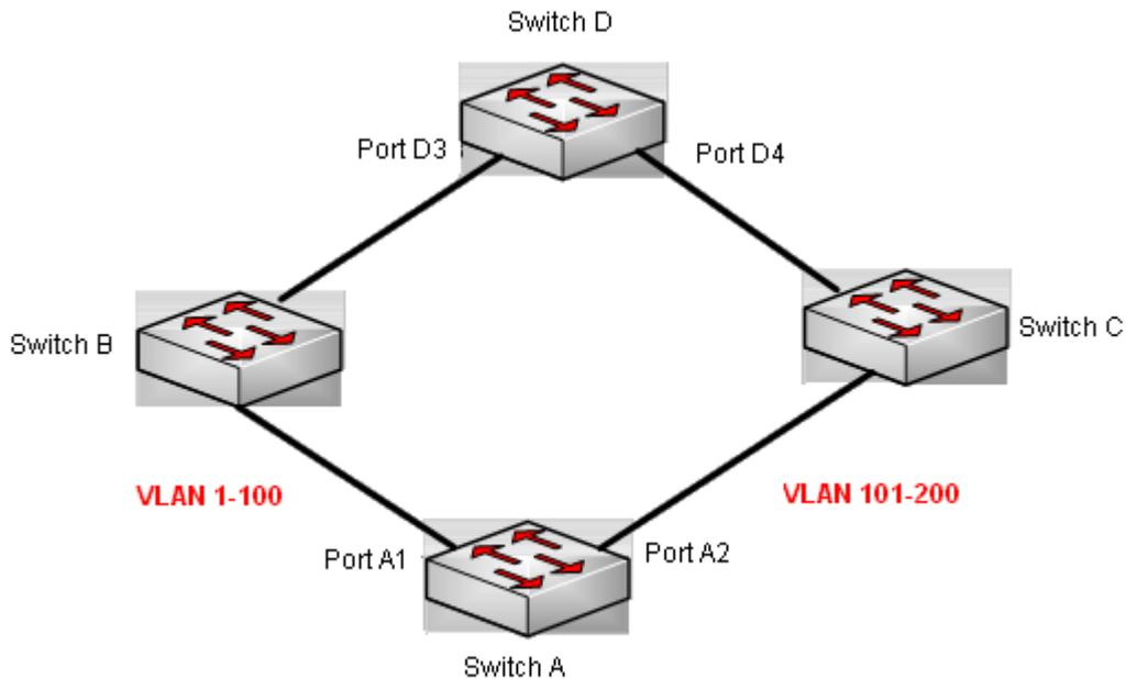
Figure 6-14 VLAN load balance
