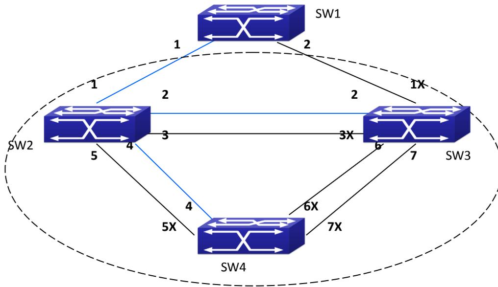
Figure 6-3 The Topology Of the Instance 0 after the MSTP Calculation
