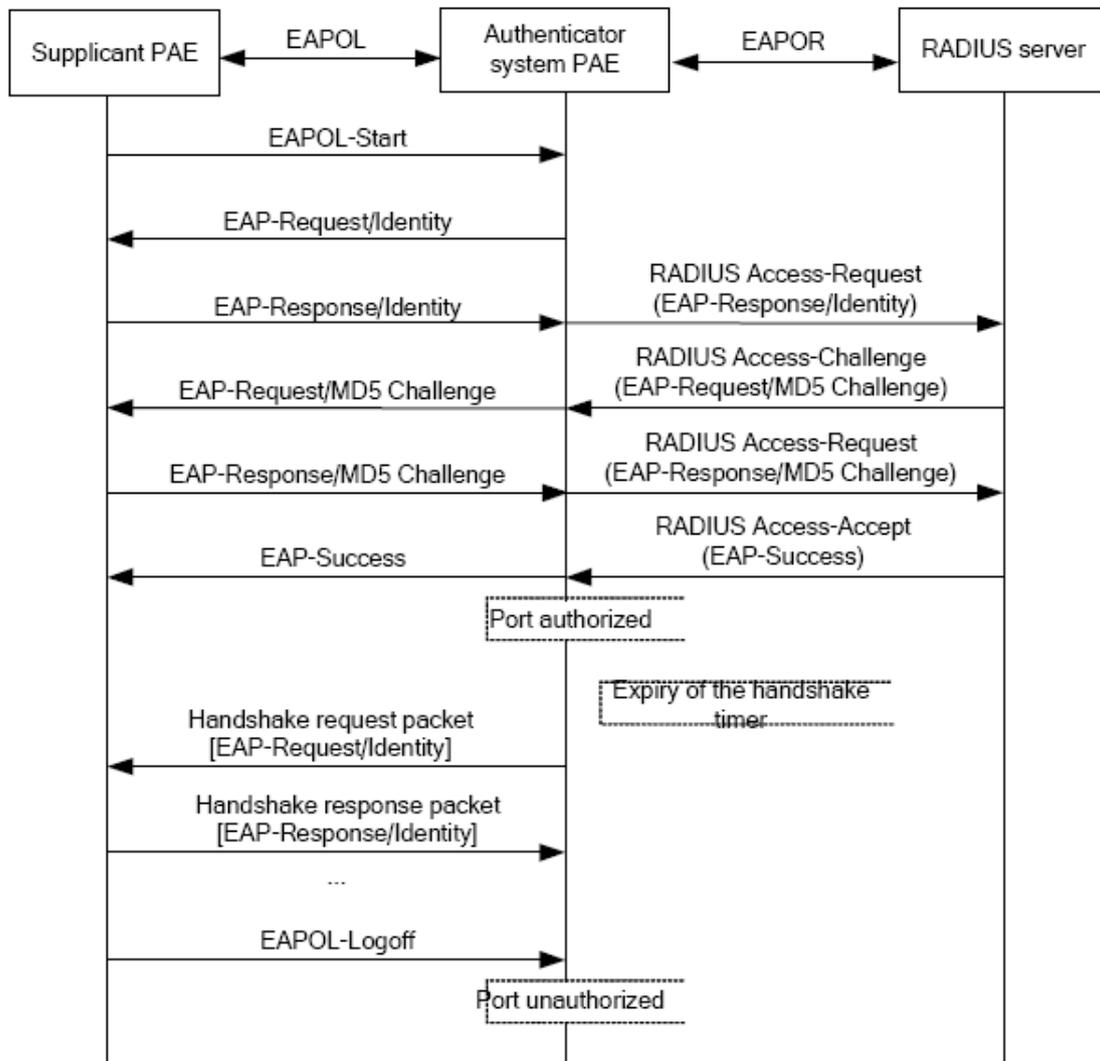
Figure 5-9 the Authentication Flow of 802.1x EAP-MD5
