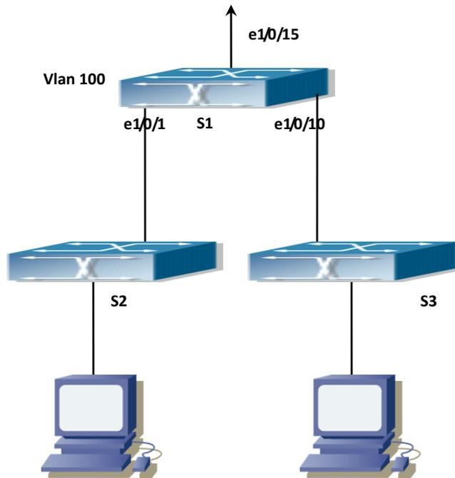
Figure 2-2 Typical example of port isolation function
