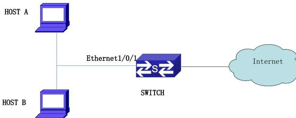
Figure 2-17 Typical topology chart for port security
