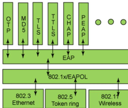
Figure 5-8 the Protocol Stack of EAP Authentication Method
