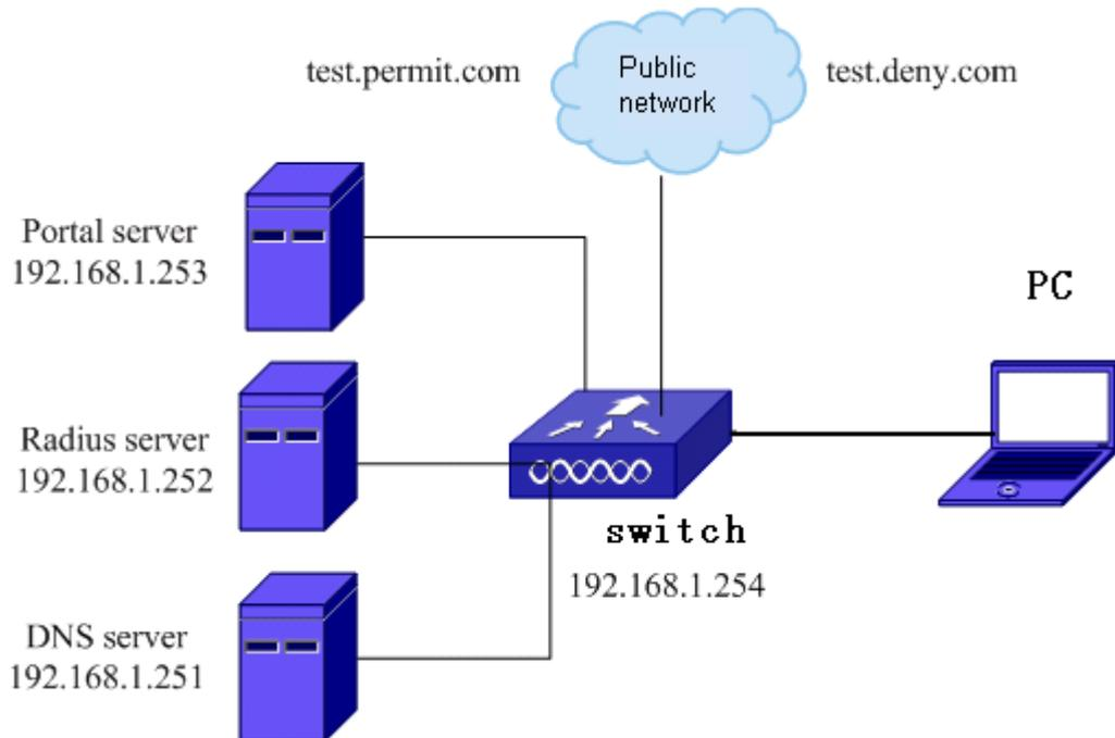
Figure 5-32 http-redirect-filter function case
