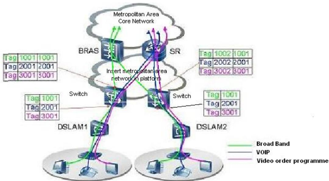
Figure 5-48 exible QinQ application topology
