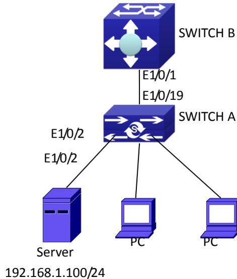
Figure 3-1 ARP scanning prevention typical configuration example
