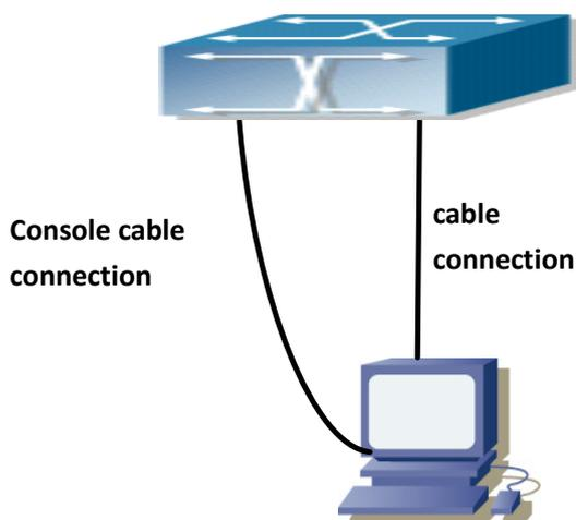
Figure 1-13 Typical topology for switch upgrade in BootROM mode
