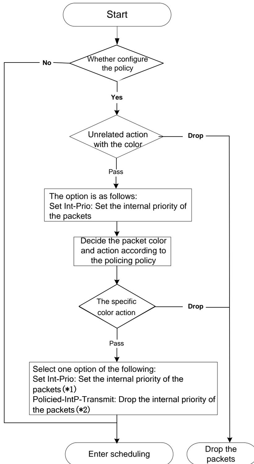
Figure 5-45 Policing and Remarking process
