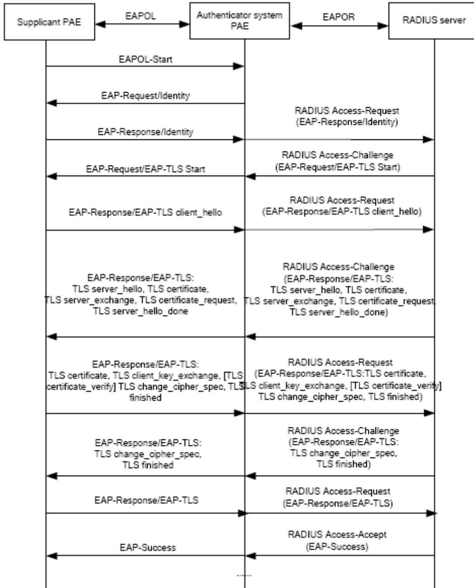
Figure 5-10 the Authentication Flow of 802.1x EAP-TLS
