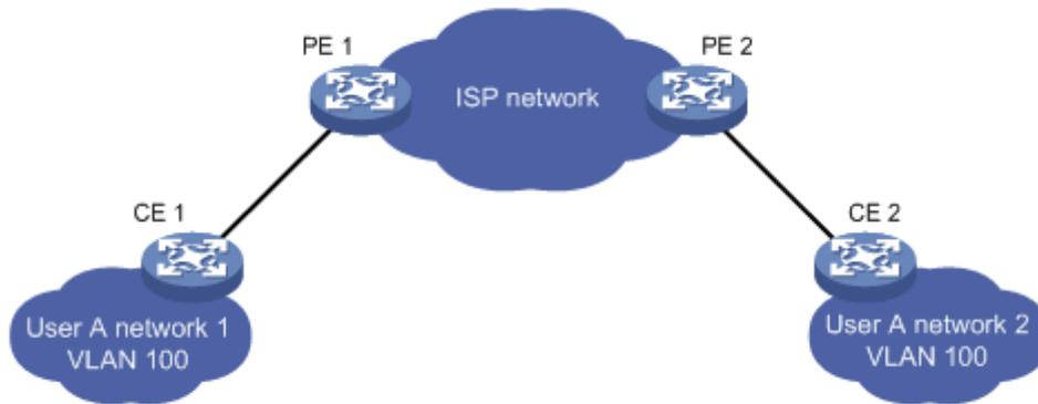
Figure 2-13 BPDUs Tunnel application environment
