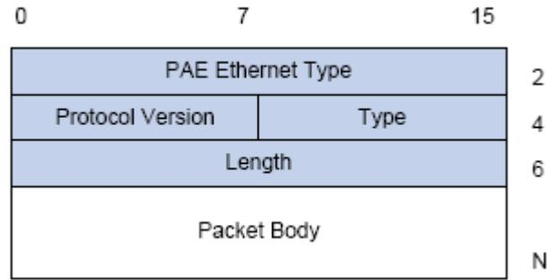
Figure 5-3 the Format of EAPOL Data Packet
