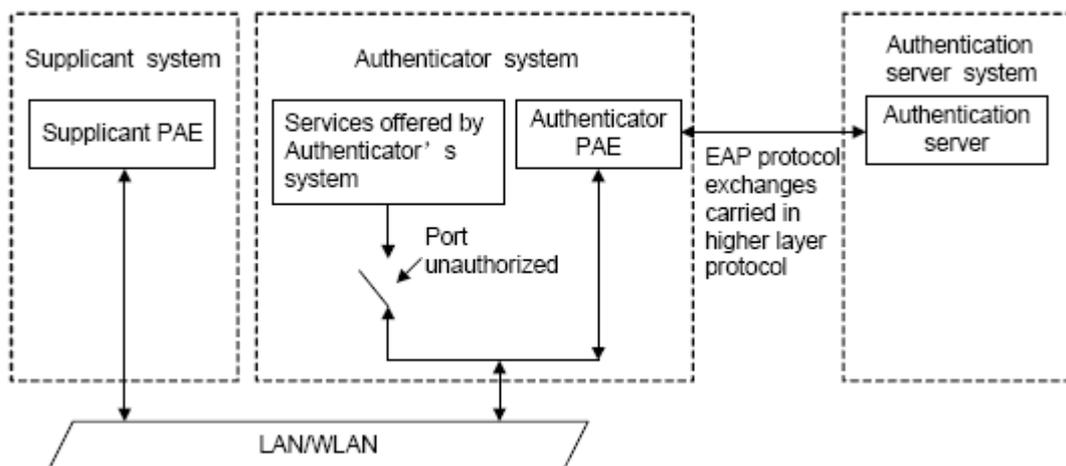
Figure 5-1 The Authentication Structure of 802.1x
