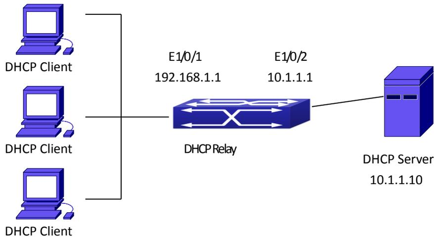
Figure 3-6 DHCP Relay Configuration
