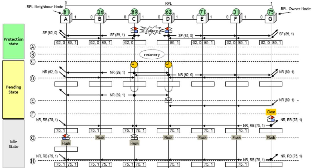
Figure 6-8 Non-revertive switch fault restoration of single link
