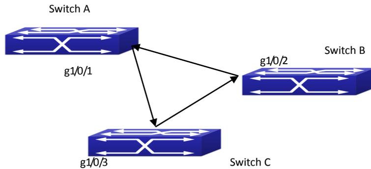
Figure 2-5 One End of Each Fiber Not Connected
