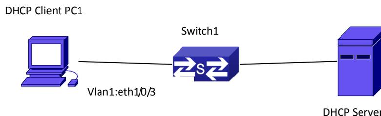
Figure 3-12 DHCP option 82 typical application example
