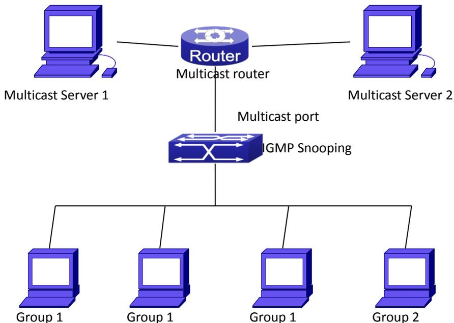
Figure 4-1 Enabling IGMP Snooping function
