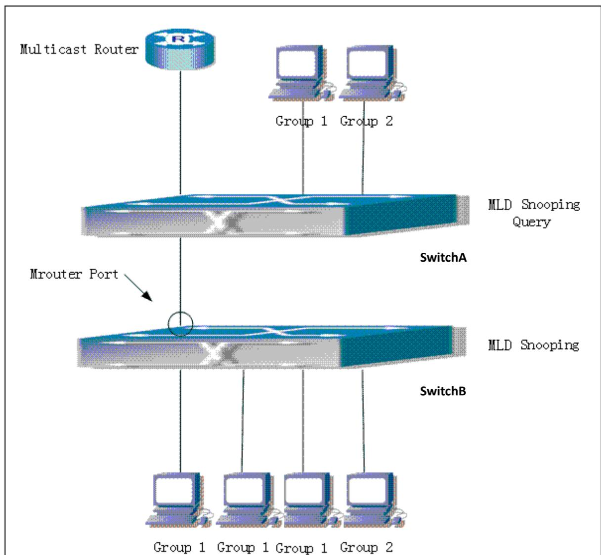
Figure 10-5 Switch as MLD Querier Function figure
