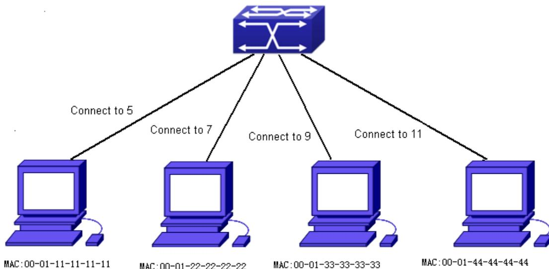
Figure 2-31 MAC Table typical configuration example
