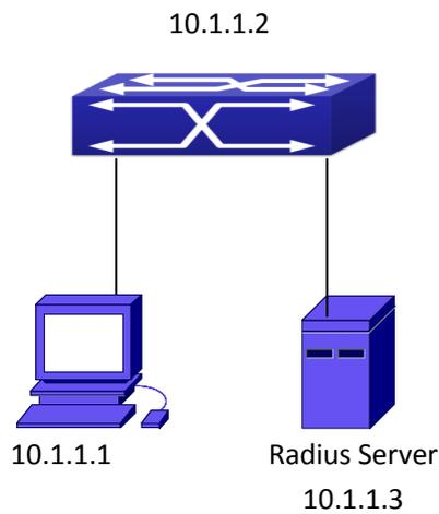
Figure 5-22 The Topology of IEEE802.1x configuration
