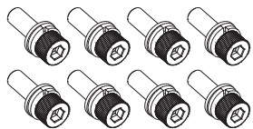
HEXAGON SOCKET HEAD SCREW (HEX S6, M8 X L25)
