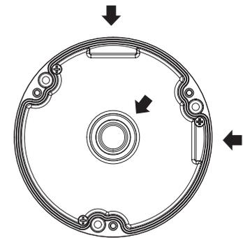
3 Attach the case-bottom to the mount bracket.
