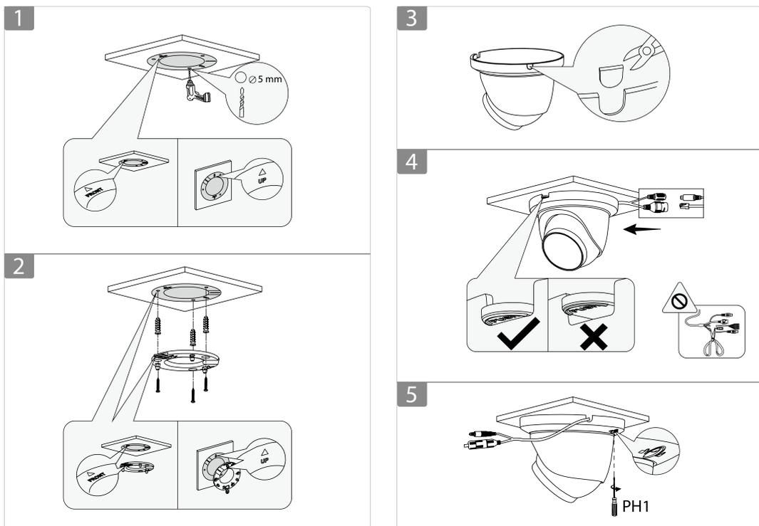
Figure 3-4 Cable going through the mounting surface
