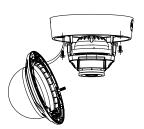
2. Reinstall the bubble assembly to the dome.
