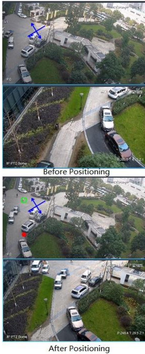
Figure 3-115 3D positioning (Zoom in after positioning)
