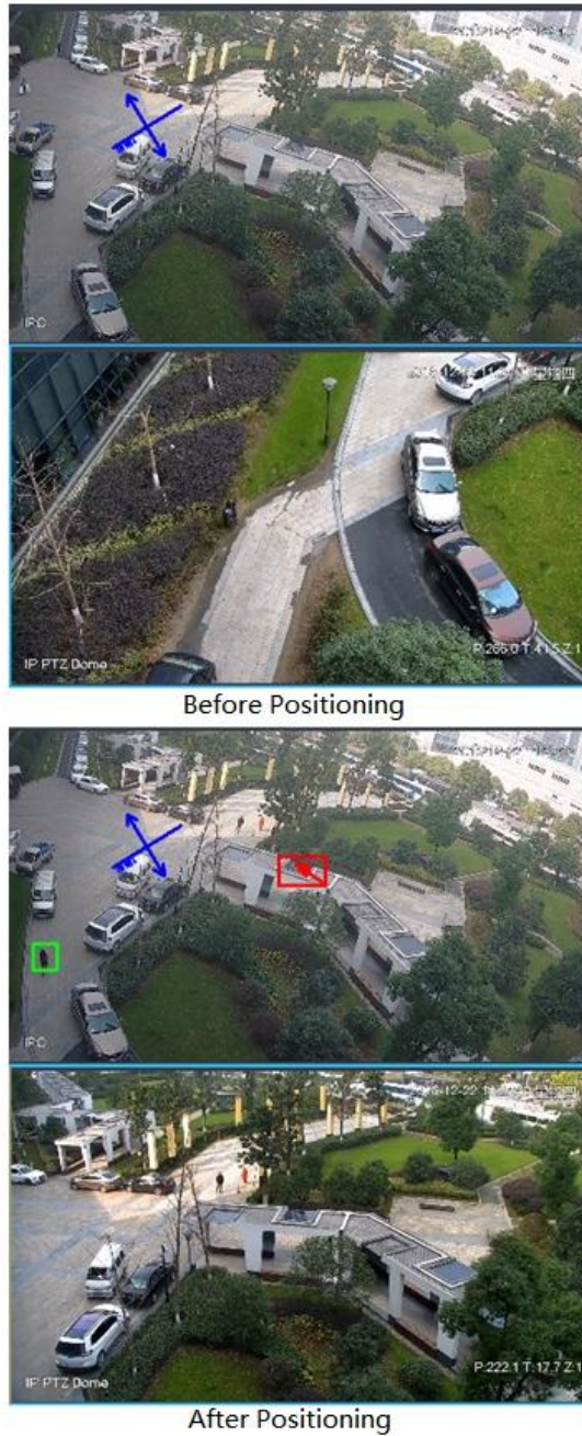
Figure 3-116 3D positioning (Zoom out after positioning)
