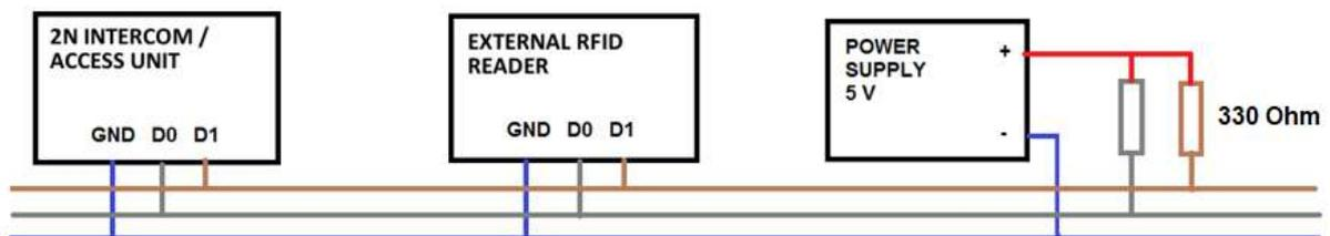
Recommended reader wiring diagram with OC output
