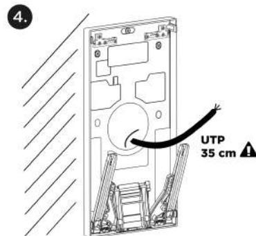
Drill chassis anchoring holes on a proper place. Use the chassis itself as a template to maintain the horizontal level and carry the cabling at the bottom edge of the cable hole. The recommended length of the accessible cables is 35 cm (1).
