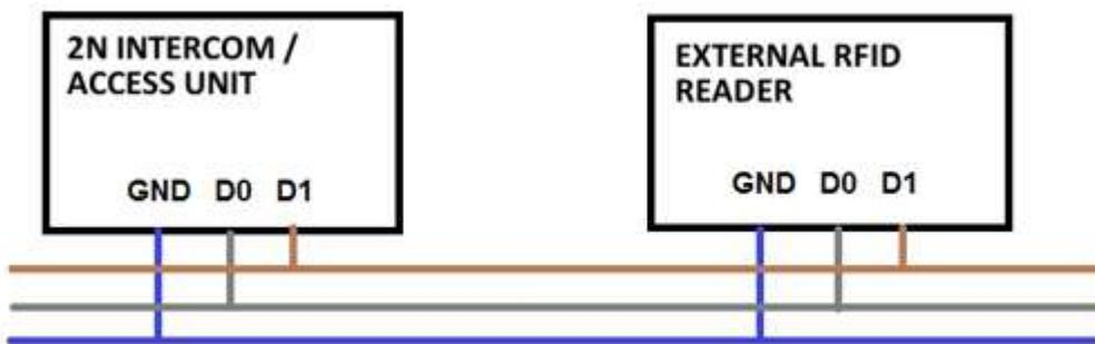
Recommended reader - bus driver wiring diagram
