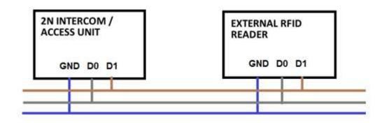
Recommended reader - bus driver wiring diagram
