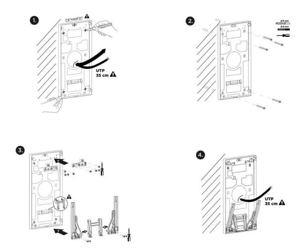
Drill chassis anchoring holes on a proper place. Use the chassis itself as a template to maintain the horizontal level and carry the cabling at the bottom edge of the cable hole. The recommended length of the accessible cables is 35 cm (1).
