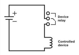
Wiring diagram for breaking of the electric circuit of the device to be controlled
