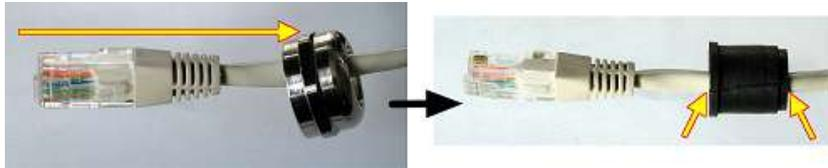
4. Replace the cover onto the sealing.
