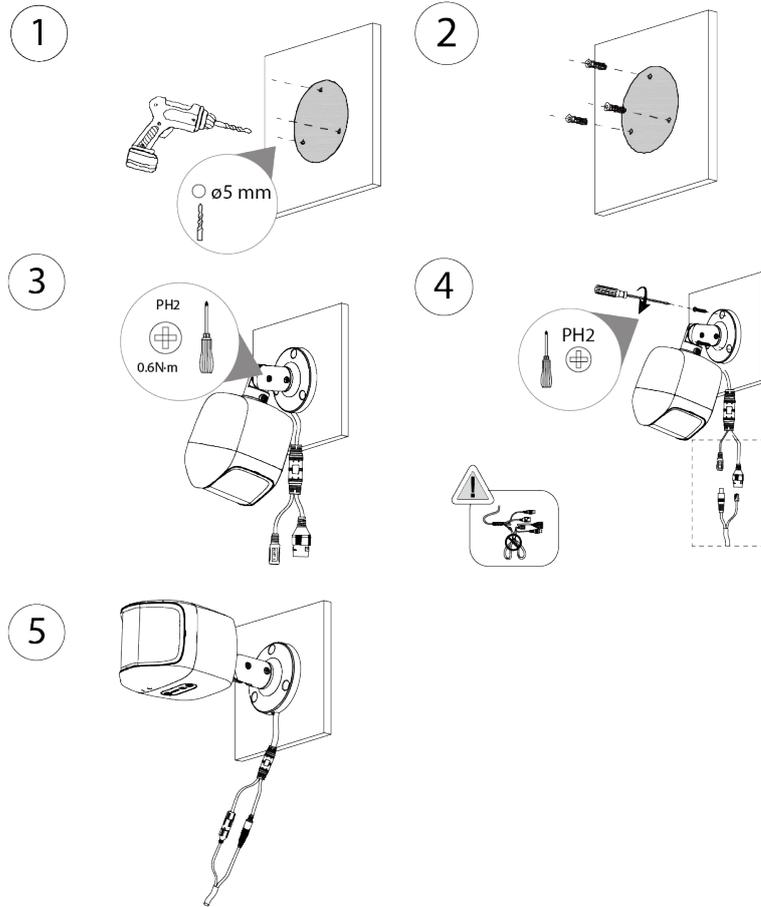
Figure 3-6 Cable going through the mounting surface
