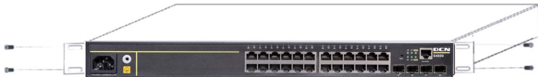
Fig 2-1 Fasten the Brackets to the Switch
