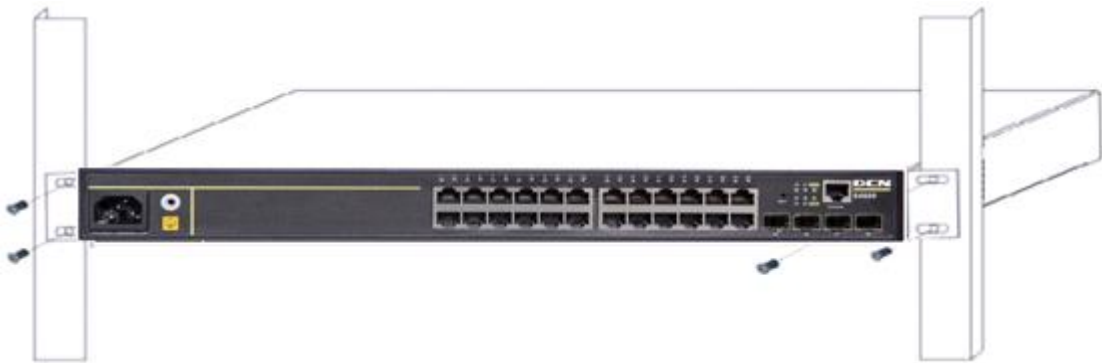
Fig 2-2 Fasten the Switch to the Rack
