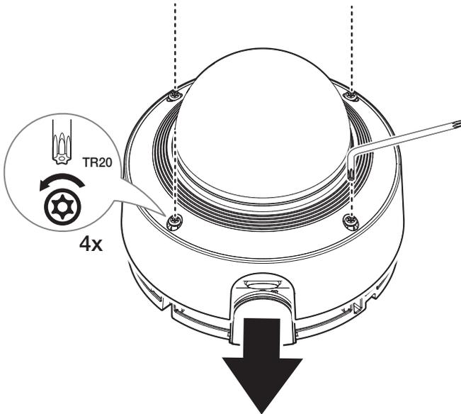
2. Use the provided Torx L wrench to turn the mount plate screws counterclockwise to release the camera body.
