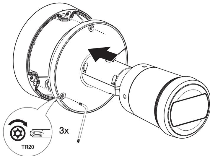
4. Adjust the camera direction using the Torx. wrench.
