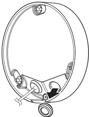
2. Mount the cable bushing of the provided audio/alarm cables to the Bottom cover.
