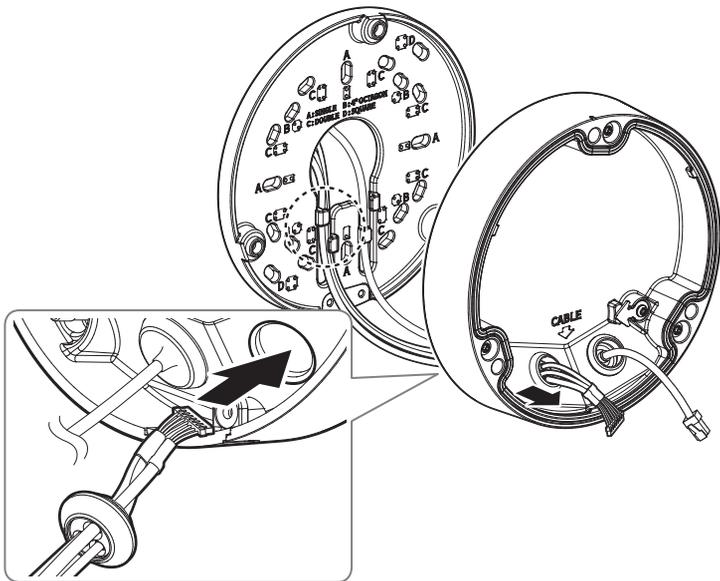
3. Join the Mount plate with the Bottom cover.
