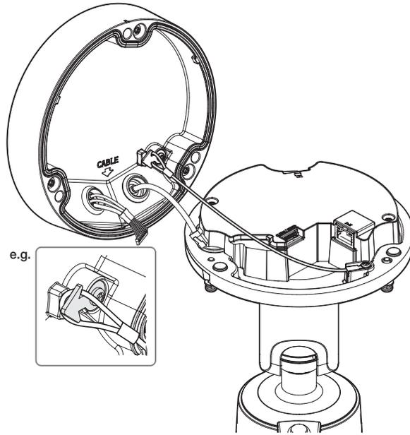
2. Connect the network cable and audio/alarm cable connector to each port of the camera body.
