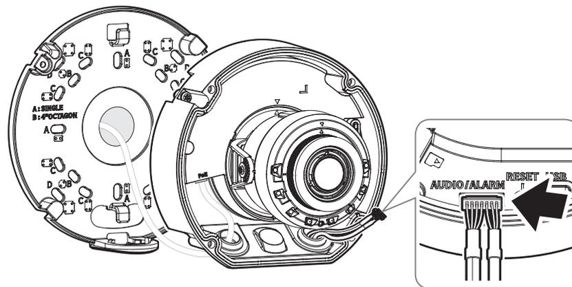
4. Join the camera body with the mount plate.
