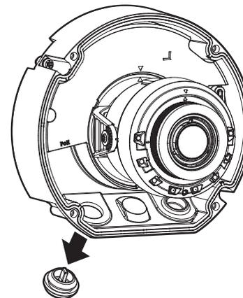
2. Remove the protruding part of the 1-hole cable bushing that was removed from the camera body.
