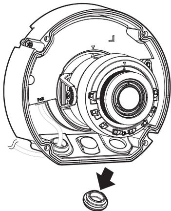
2. Mount the cable bushing of the provided audio/alarm cables to the camera body.
