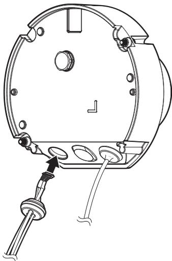
3. Connect the audio/alarm cable connector to the audio/alarm cable port of the camera body.
