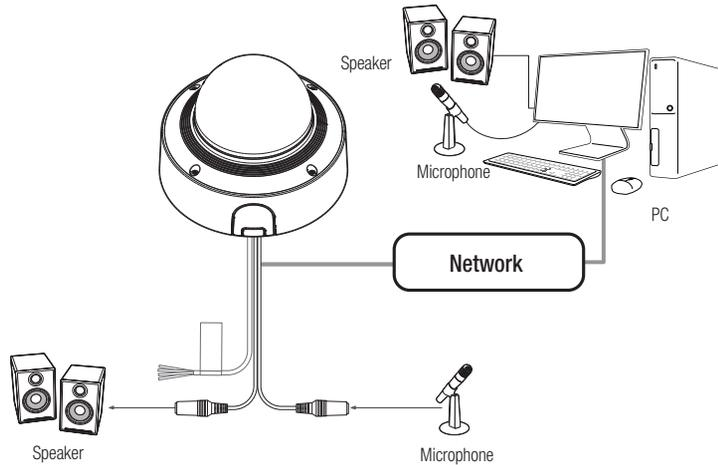
1. Connect the MIC port of the camera with the microphone or LINE OUT port of the amplifier that the microphone is connected to.
