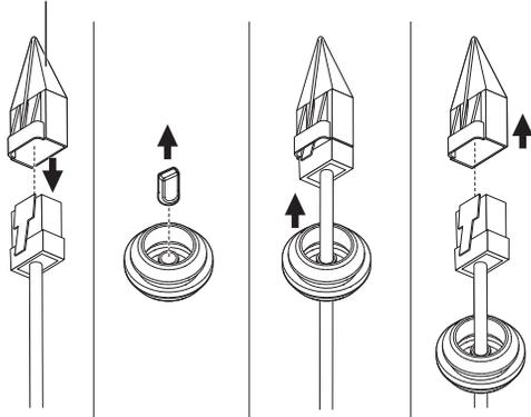
4. For waterproof protection, pull down the cable below the cable bushing as shown in the figure below.
