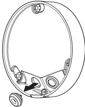
2. Remove the protruding part of the 1-hole cable bushing that was removed from the Bottom cover.
