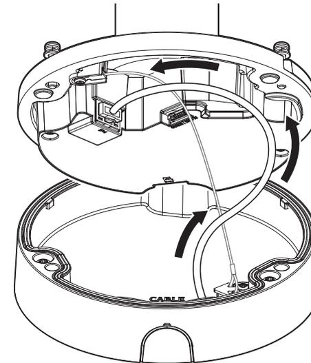
3. Join the camera body with the Bottom cover.
