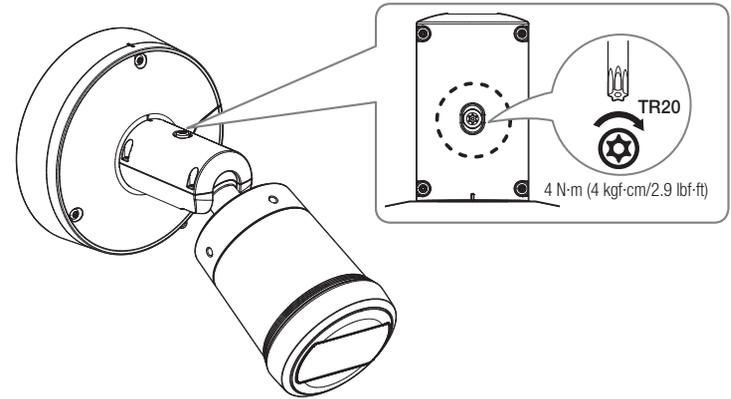
6. Use the sunshield mounting screws and tooth washers to join the sunshield to the camera body.
