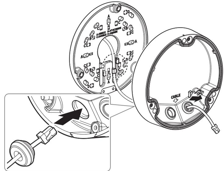
[Installing audio/alarm cables]
