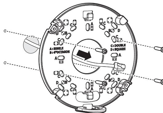
☑ ■ When connecting the cable through the side, remove the wiring hole cover first before doing so.
