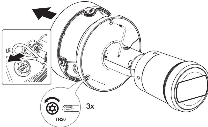
2. Remove the fixing tape from the bottom cover and mount plate, and then remove the mount plate.
