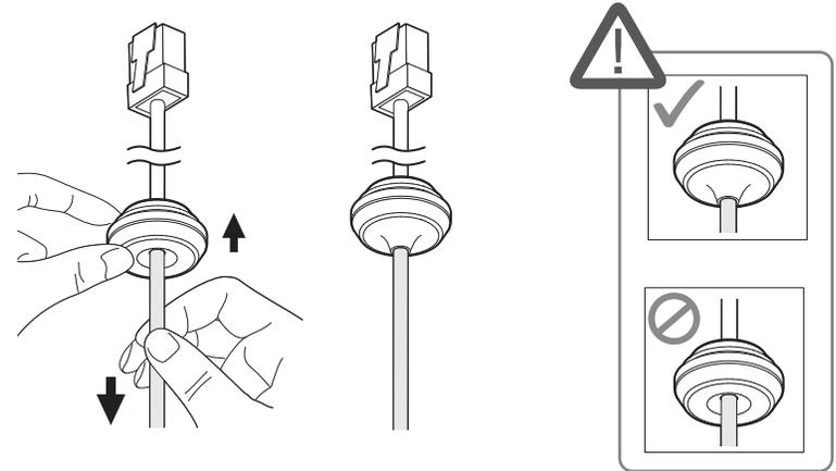
5. Insert the cable bushing of the network cable into the bottom cover.
