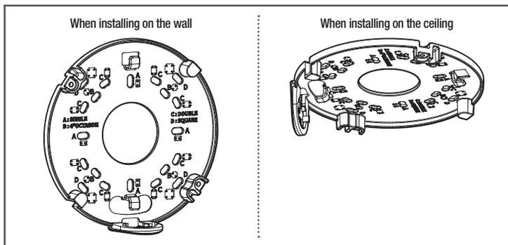
1-2. Fix the mount plate using appropriate screws.
