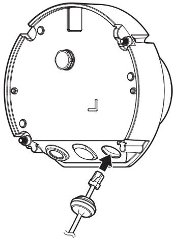
6. Connect the network cable connector to the PoE port of the camera body.
