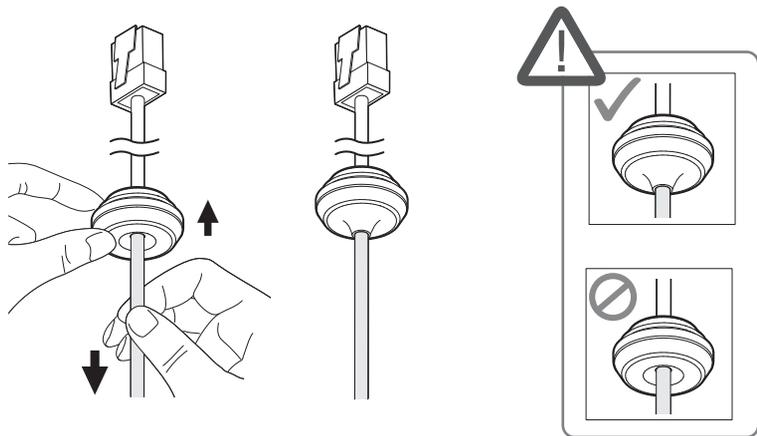
5. Insert the cable bushing of the network cable into the camera body.
