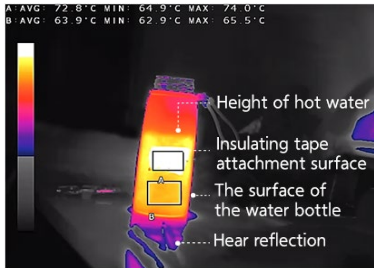
[Figure 21. A difference in thermal imagery according to emissivity when filling up hot water in the water bottle]
