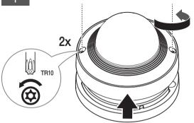
Directly installing on wall/ceiling
