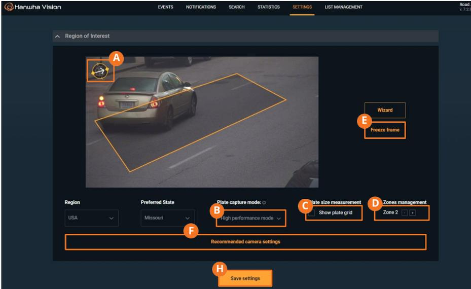
**A** Set the **vehicle direction\***: align the arrow in parallel to the vehicle direction vector, pointing the arrow towards the chosen standard vehicle direction.
