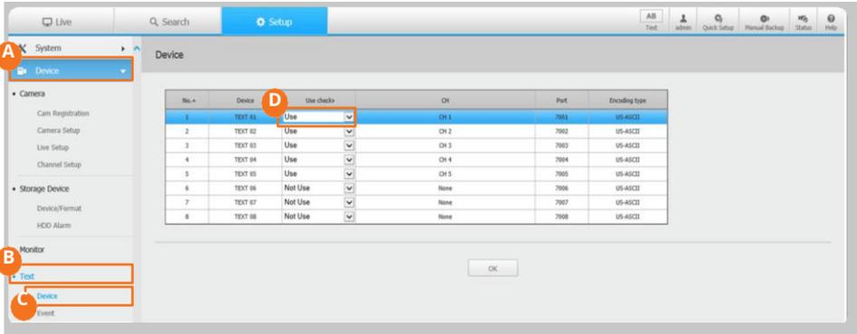
Check the NVR settings to obtain corresponding Port number in **A** Device; **B** Text ; **C** Device setting (by default port 7001 for CH 1, 7002 for CH 2, etc.)
