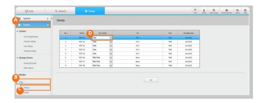
Check the NVR settings to obtain corresponding Port number in 🛕 Device; BText; Device setting (by default port 7001 for CH 1, 7002 for CH 2, etc.)
