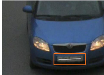
Improper focus settings. Adjust the lens.
