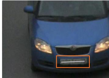
Improper focus settings. Adjust the lens.
