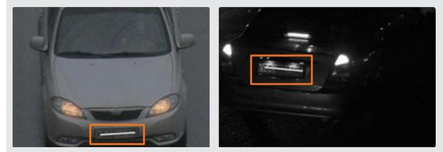
Insufficient light. Adjust exposure settings or provide additional lighting.
