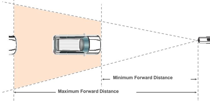
Camera in 4K mode can cover up to 3 road lanes. The FullHD mode can cover up to 2 lanes.
