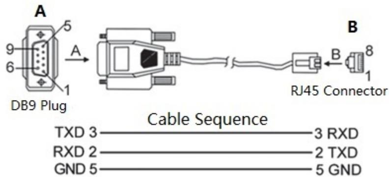
One end of RJ45 DB9 cable is RJ45 connector, which needs to be inserted into the console port of the device. And the other end is DB9 plug, which needs to be inserted into the computer controlling 9-pin serial port.
