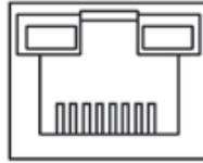
See Figure 3-4 for console port. The switch console port and computer controlling 9-pin serial port are connected with RJ-45-DB9 cable. You can call the console software of the device by operating the superterminal software of the Windows system for device configuration, maintenance, and management.
