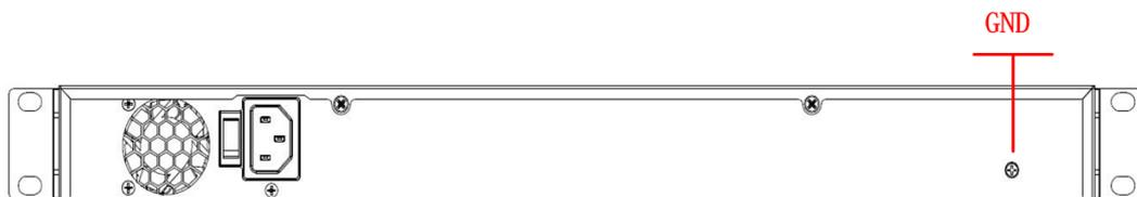
Normal GND of the device is the important guarantee for device lightning protection and anti-interference. You should connect the GND cable before powering on the device, and power off the device before disconnecting the GND cable.
