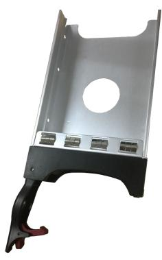
$\underline{\text{Step 3}}$  Put the HDD into the disk box and fasten the screws on both sides of the box.
