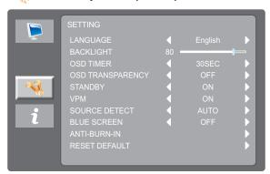
3. Press ▲ / ▼ to select an option and press 2(AUTO) to enter its submenu.
