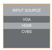
Press the ▲ key continuously to select the desired input source. Then press the 2 (AUTO) key to confirm or wait until the source menu disappears from the screen automatically. The available input options include "CVBS", "HDMI", and "VGA".
