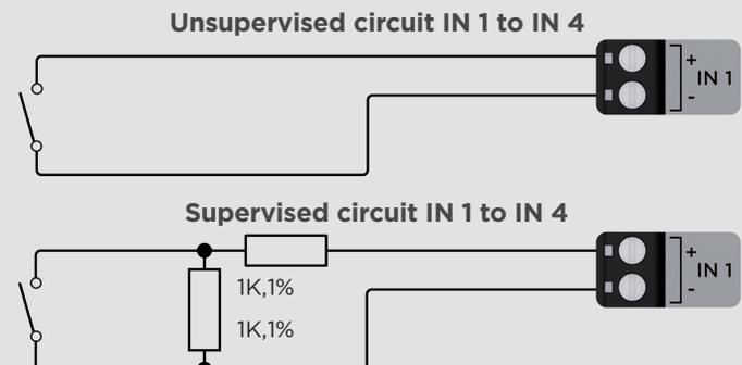
**Note:** The input circuit wiring configurations shown are supported but may not be typical.
